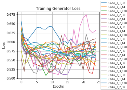
Figure 18: Generator loss for CCGANs, the first number in the name means the size of F , the second number the depth D and the last number batch size B .
